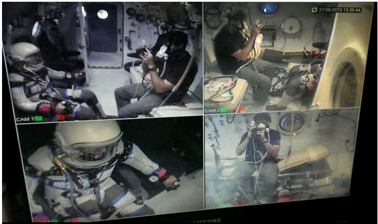
FIGURE 2. Pressure Garment Operator Test Subject in Trykkammer, Monitored by Closed-Circuit Video During Depressurization Test. Photo courtesy of Kristian von Bengtson, Copenhagen Suborbitals.
